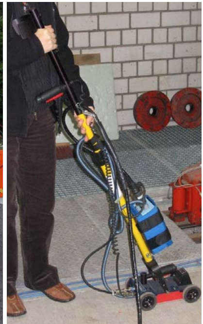
Fig. 3 - 1,5 GHz GSSI dipole antenna : measuring in test pit
