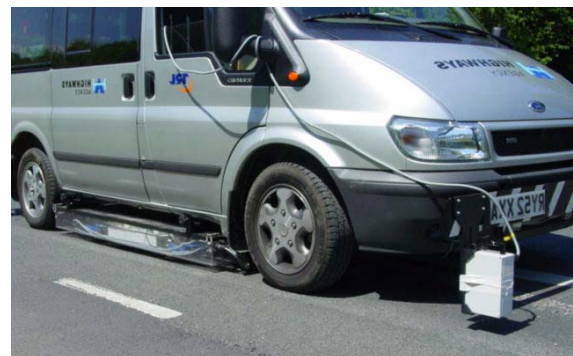
Fig. 6 - Four-channel system used in TRL: attachment to measuring car Harris (photo TRL)
