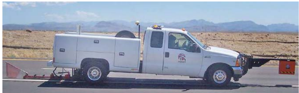
Fig. 1 - GSSI integrated system: measurement of bearing capacity by FWD and diagnostics by GPR
