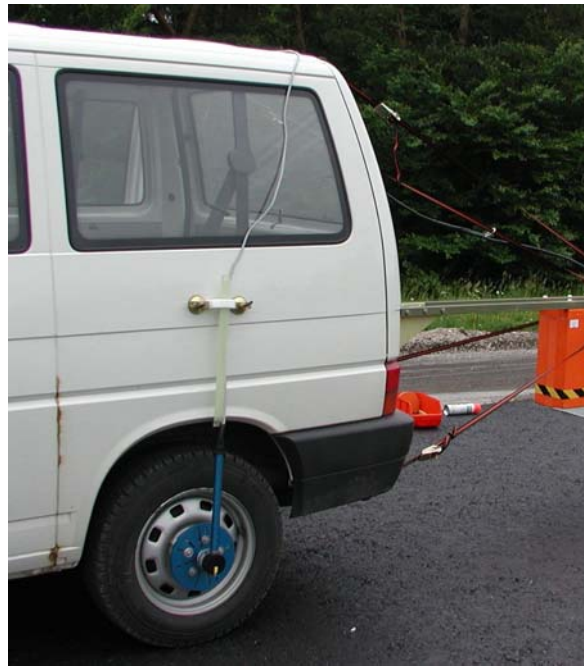
Fig. 2 - 2 GHz GSSI horn antenna : attachment to the measuring car
