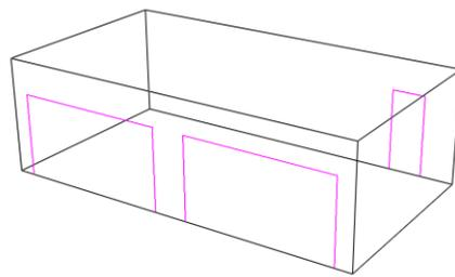
Figure 5. Two-zone model for the analysed space
