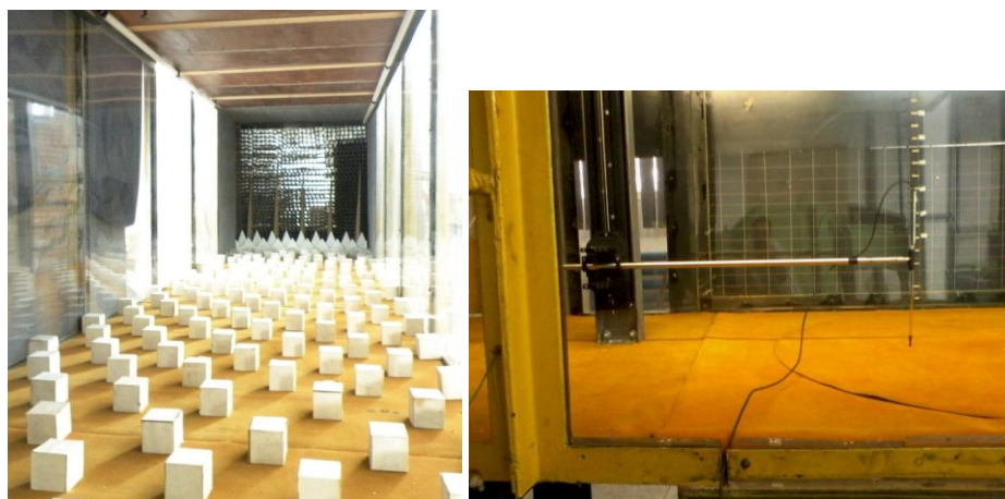
Fig. 3 View inside the BLWT: a) system for generating the turbulence of the flow over an II category of terrain; b) equipment for acquisition of wind velocity
