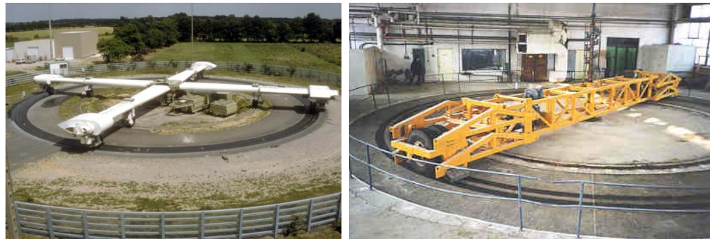
Fig. 3 Circular ALT facilities [9]
