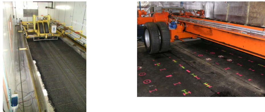
Fig. 4 Linear ALT Facility[9]
