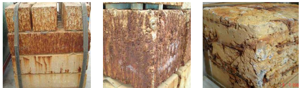
a) overall view of the samples b) view of corroded RCC sample with recycled fibres c) view of corroded RCC sample with industrial fibres
