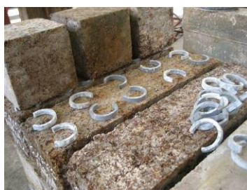
a) specimens being positioned in the frame before corrosion
