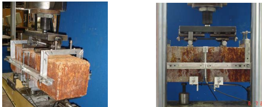
Figure 8 – Specimen in the flexural test.
