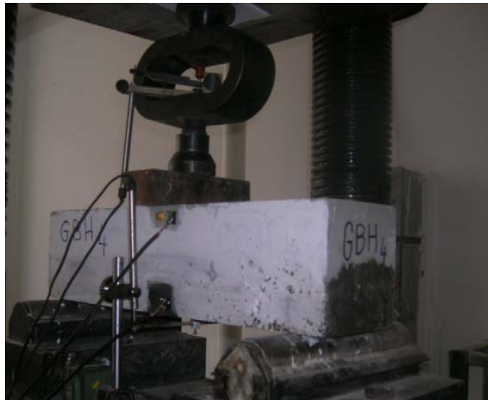
Figure 2. Three point loading test of the hybrid beams
