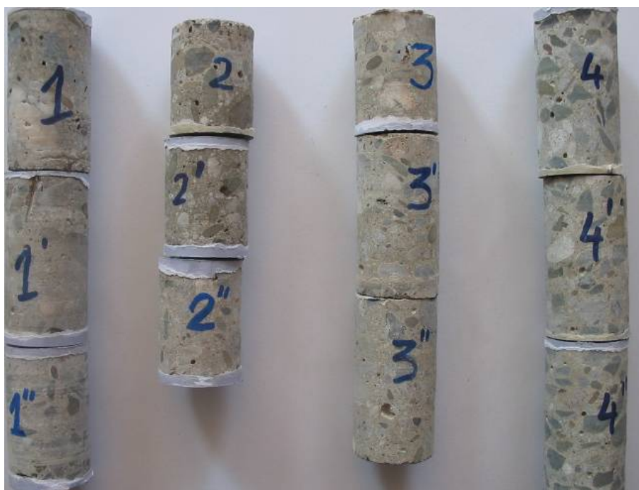
Figure 6. Concrete test rods from the superstructure
