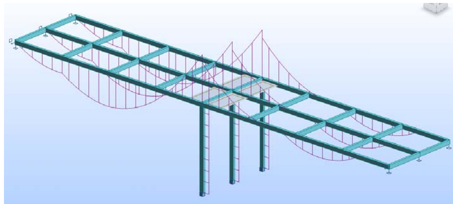
Figure 10. Bending moment from additionally loading from the hydraulic jacks and permanent load
