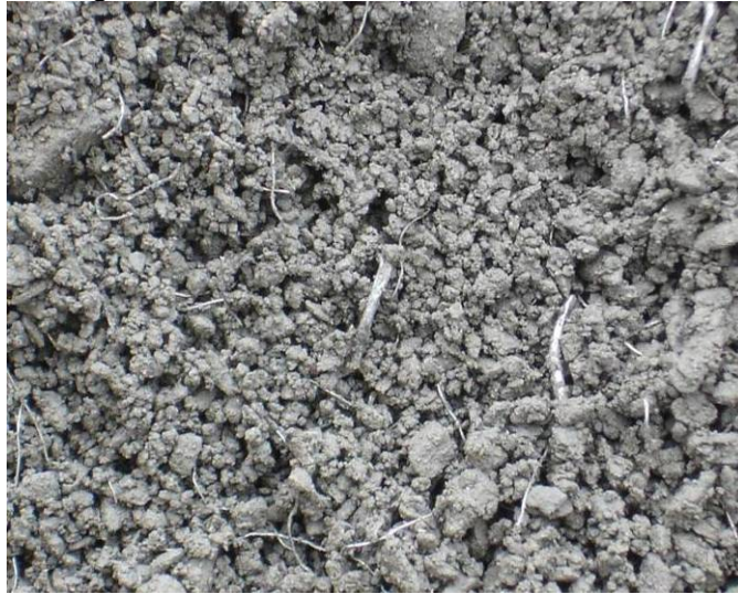
Figure 5 – SFR-RCC produced in an industrial pan mixer
