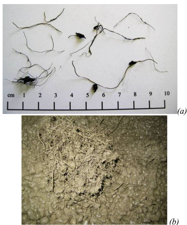
Figure 4 – (a) Irregular steel tyre-cord fibres, produced from the shredding of post-consumer tyres (b) Fibre balling in wet-mix concrete
