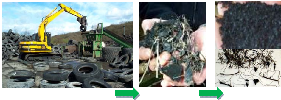
Figure 1 - Mechanical shedding of post-consumer tyres: recovery of rubber and steel
