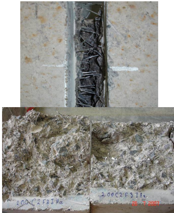
Figure 10 - Fibre pull-out of a cracked SFR-RCC specimen
