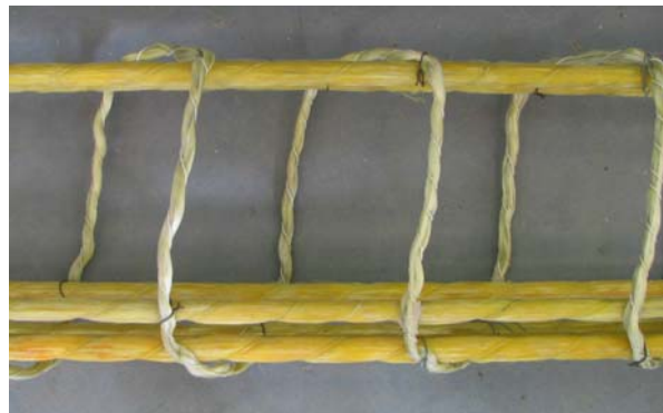
Figure 5. Shear reinforcement shaped into spiral
