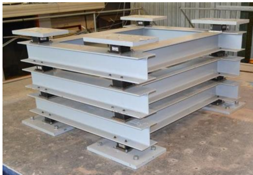
Figure 2. Multi-stage isolation system with elastomeric bearings
