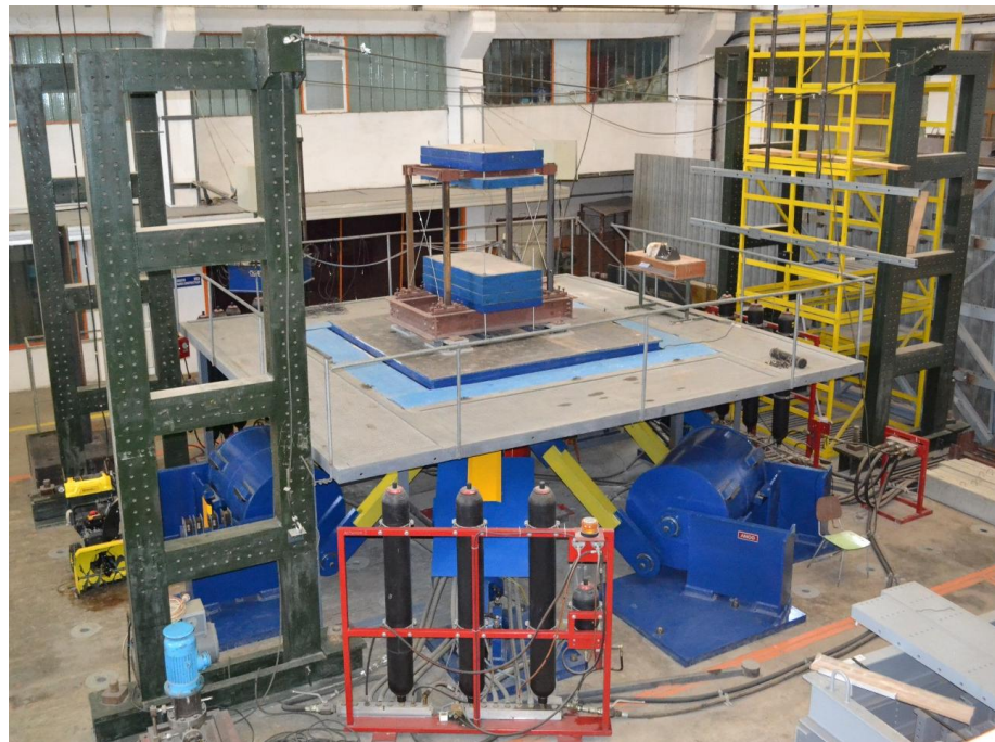
Figure 1. The base isolated structure on the shaking table
