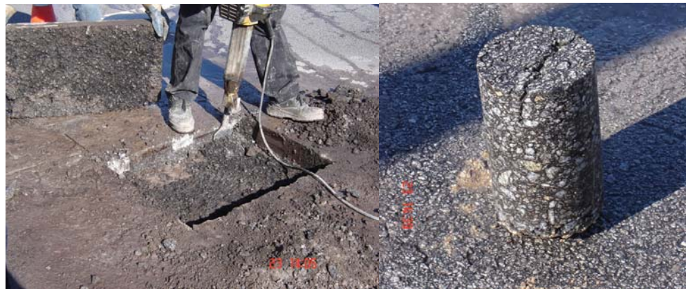
Figure 4. Coring: a) splitting of the asphalt layer; b) top-down cracking
