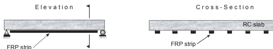
Figure 3. FRP strengthening of one-way simply supported plate: a- elevation; b- cross section
